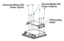
An additional four screws (not included in the kit) are required to mount the display on a VESA rack. For this purpose, use M6 screws with a length between 10 and 12 mm.
