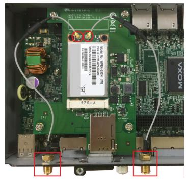
Pass the antenna mount's threaded connection ring through the mounting hole, hold the locking washer against the rear panel and secure the antenna connector by tightening the nut onto the threaded protection ring.
