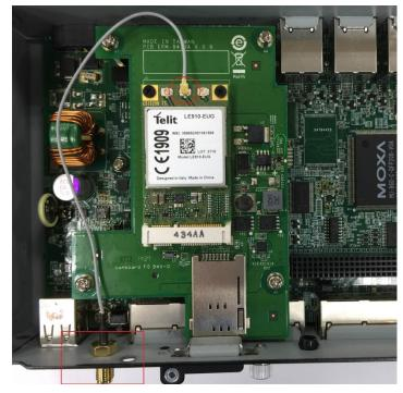
4. Pass the antenna mount's threaded connection ring through the mounting hole, keeping the locking washer against the rear panel face. Secure the antenna connector by tightening the nut onto the threaded protection ring.
