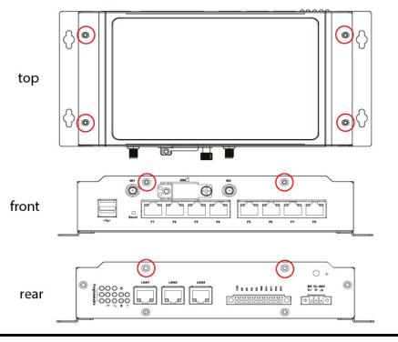
**NOTE** The top cover comes loose only after you have removed all eight screws as indicated in the diagrams.
