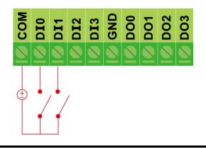
**NOTE** If you are using wet contacts, you must connect "COM" to power.
