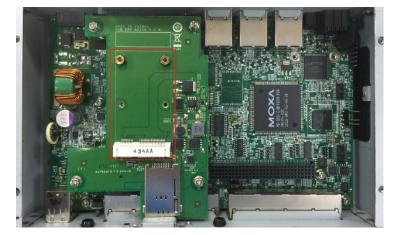
2. Insert the module in the socket and fasten the two black screws on the module.
