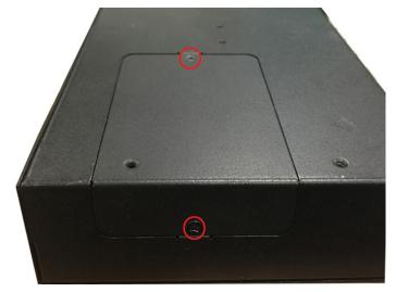
2. Remove the cover to access the SD-card slot and the mSATA socket.  $$\rm mSATA$$
