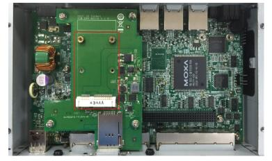
2. Insert the module into the socket and fasten the two black screws on the module.
