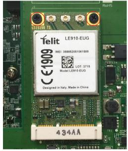
3. Attach one end of the cellular cable on the central connector, and then connect the other end of the cable on the W1 hole on the front panel of the computer.Remove the antenna hole protection cover before you do so.
