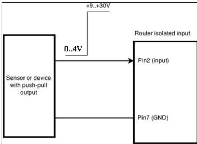
The signal source resistance should be less than 100Ω.
